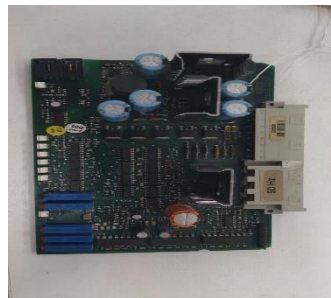
Voltage monitoring card (AC338 - Old type GZK)
