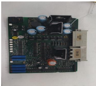
Voltage control card (AC338 - Old type GZK)
